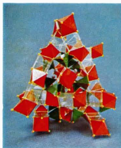
Fig. 23. A polyhedral model of the garnet structure. Red octahedra and transparent trigonal prisms form rods packed in b.c.c. rod packing. The rods are joined by green SiO_4 tetrahedra. Some of the large cation sites are shown by grey balls. The small yellow balls represent oxygen atoms.
